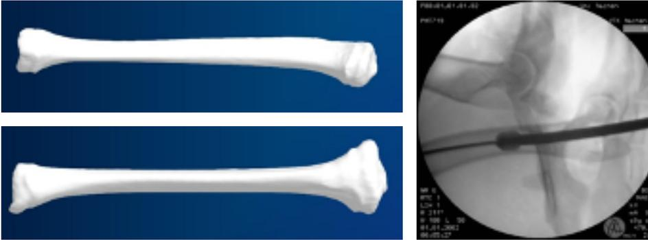
Figure 4: Sample sheep bones from additive manufacturing (left) and X-ray image from a sheep cadlab with master scale for dimension reference.
