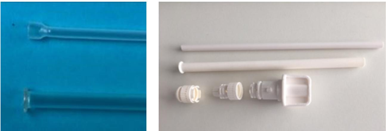
*Figure 2: The extruded cannulas for the BONEBANK harvesting device. The tubes (inner and outer cannula) are manufactured from polypropylene (PP) and temperature-formed at their ends (see left) to allow glue-free assembly with the cannula adapter parts (shown on the right).*
